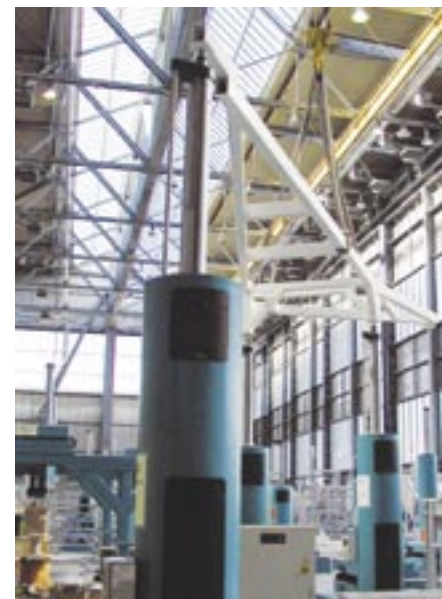
ON-SITE FABRICATION AND WELDING 787 mandrel handler manufactured to Aerospace industry standards.
