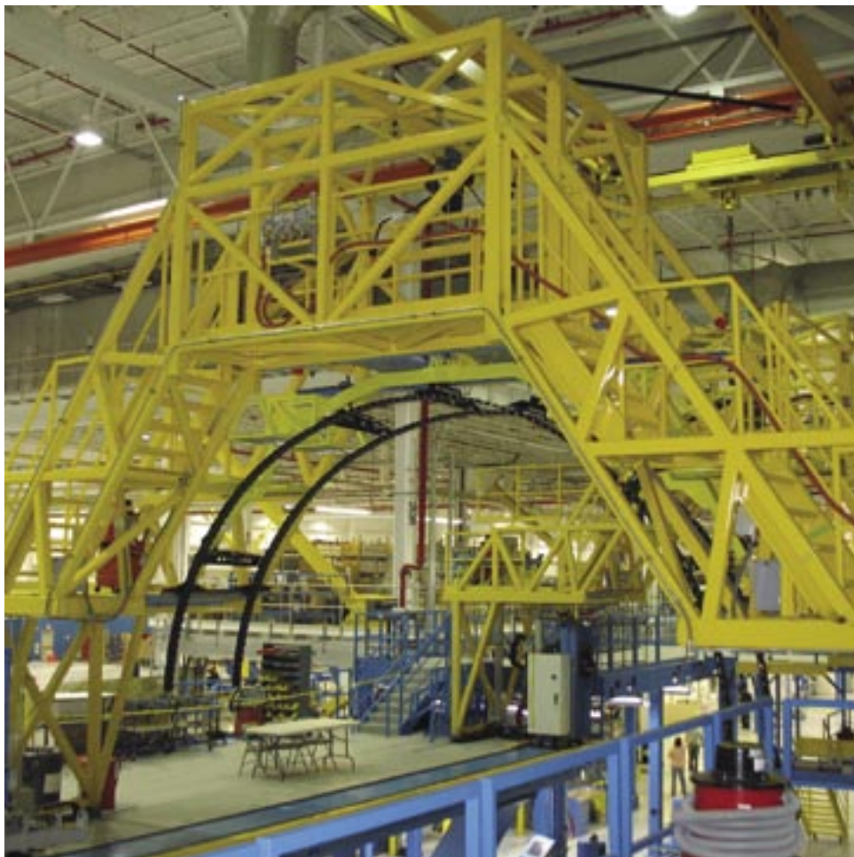
FIGURE 4 ✂ Global Aeronautica 787 flexible tracks at Charleston, SC, facility.
