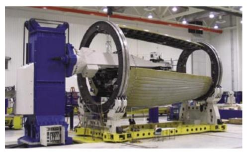
**AUTOMATED ASSEMBLY \$\times\$** For Vought, AIT delivered a mandrel assembly/disassembly system for the 787 Dreamliner Sections 47/48.
