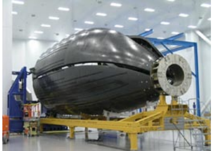
NOSE SECTION Section 41 is the 22-foot wide forward fuselage section of the 787 Dreamliner, held in position with AIT mandrel handler.
