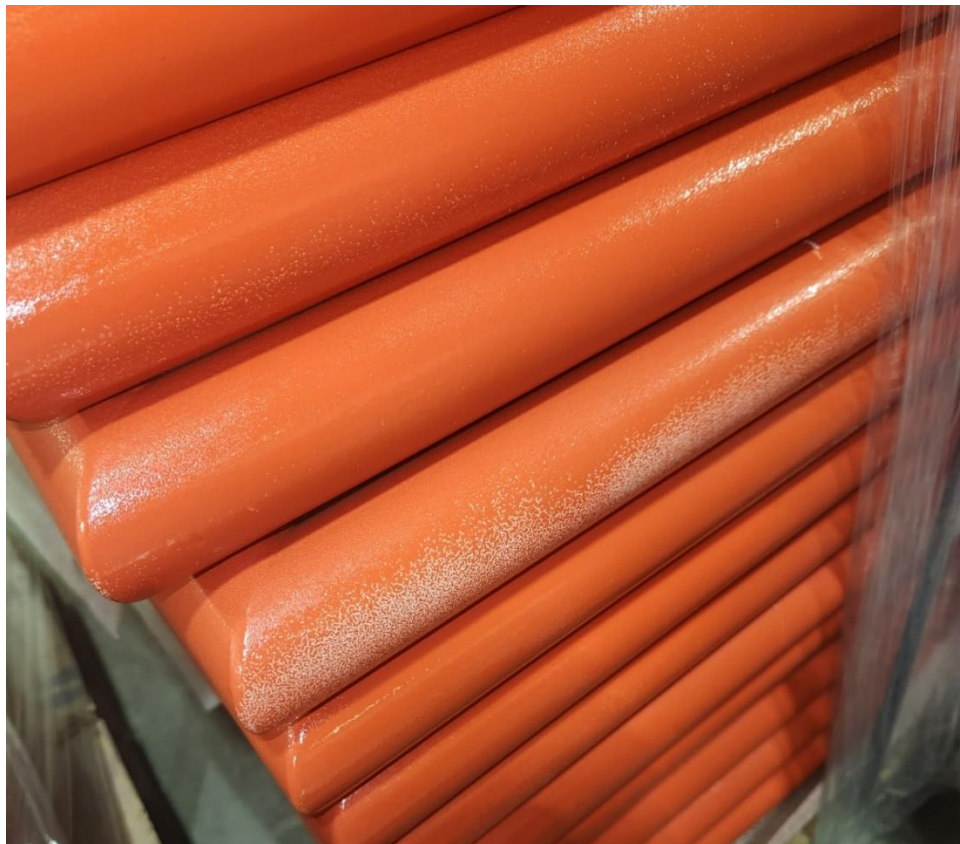
Figure 10: Unacceptable Thin topcoat / primer bleed through
