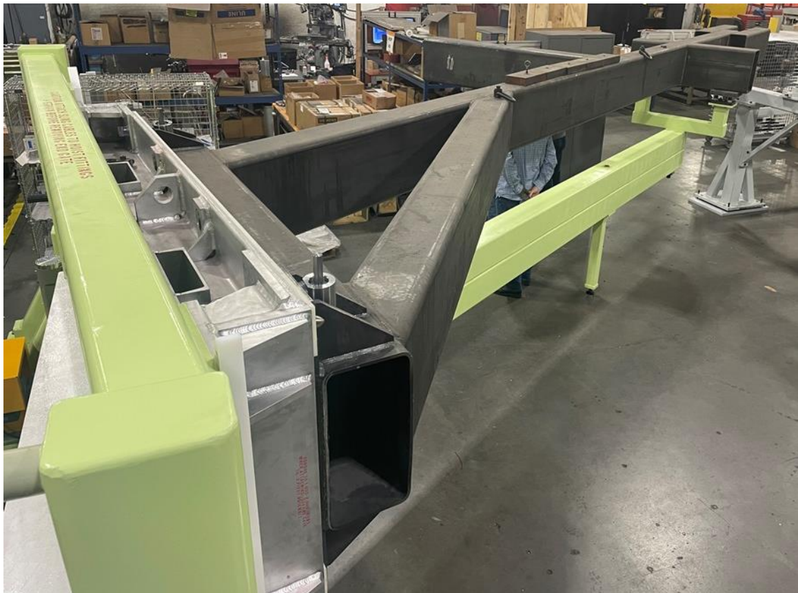
Figure 29: Show test fixtures and manufactured items used to simulate part weight (see unpainted steel weldment)
