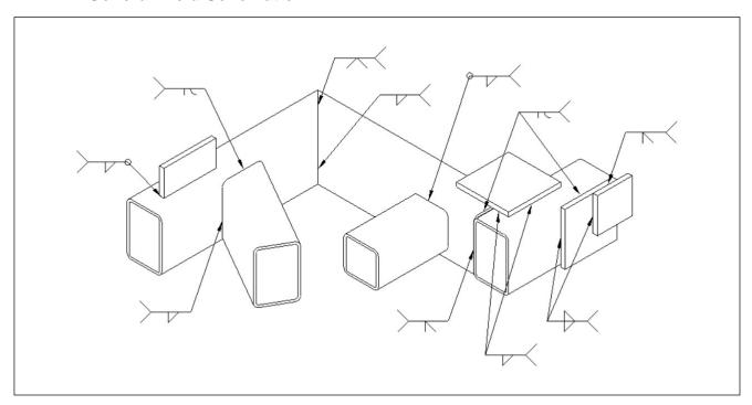
**Note:** Symbols shown above are typical for all welded joints of similar construction unless otherwise specified.
