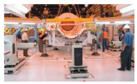
LASER-TIGHT ASSEMBLY A AIT's Automated Positioning and Alignment System used laser tracking for precision final assembly of the F-35 JSF.
