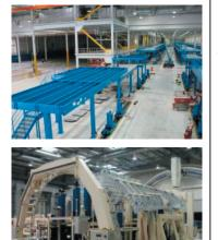
the core technology developed by AIT over more than a decade. The automated positioning and alignment system incorporated integrated laser tracking to facilitate aircraft structure alignment by locating parts and controlling aircraft geometry. AIT's integration accelerated speed to market and competitiveadvantage from curtailed cycle and ramp-up times. This was the first project of its kind to be implemented at Lockheed Martin's Fort Worth, TX, facility.
