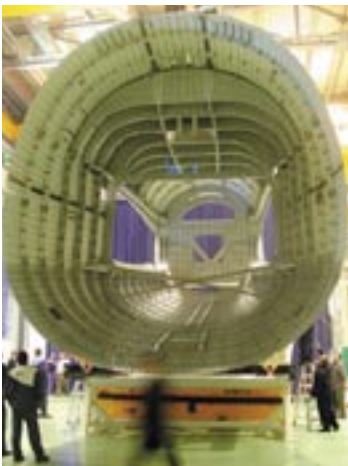
SECTION 19 Over 32' long and 28' tall at the forward end, the largest carbon fiber section at the time.
