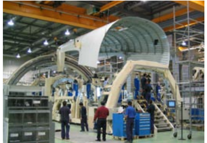
UPPER SHELL ⚡ Manipulating the Section 19 shells required AIT shell assembly systems.
